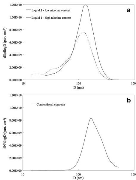
**Fig. 3.** Particle number distribution measured through the FMPS 3091 (after thermal dilution at 37 °C) of the mainstream aerosol from the Liquid 1 (a) and from the conventional tobacco cigarette (b).
