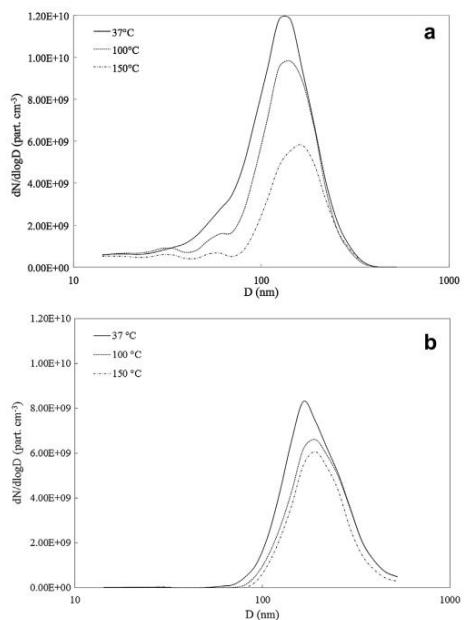
**Fig. 4.** Volatility analysis at three temperature levels (37 °C, 100 °C, and 150 °C) of mainstream aerosol generated by: (a) e-cigarette A using Liquid 1 at high nicotine content; (b) conventional tobacco cigarette.
